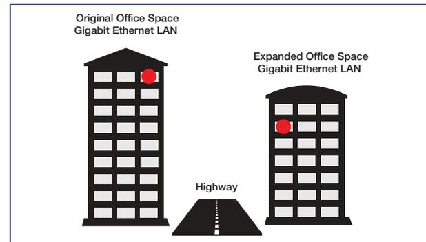
This required connectivity could have been provided by the owners of the buildings if they had established a fiber-optic cable run between the two buildings. But often there is no such level of interconnectivity between buildings. So, a second option would be to run dark fiber (i.e., privately operated optical fiber) between the two offices.
