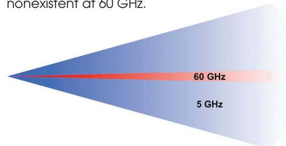
This narrow beamwidth contrasts with comparably sized 5 GHz solutions that have a beamwidth that is more than ten times as wide, thereby transmitting signals that are beyond the location of the intended receiver. In addition, a 5 GHz antenna risks the possibility of receiving interference from other 5 GHz radio links or Wi-Fi routers.
