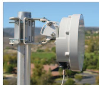
HaulPass V60s is an advanced V-Band broadband wireless solution that delivers low-latency, full-duplex Gigabit Ethernet transport speeds
