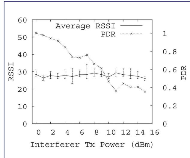
Figure 3. Wireless Link RSSI and PDR with Interference<sup>3</sup>
